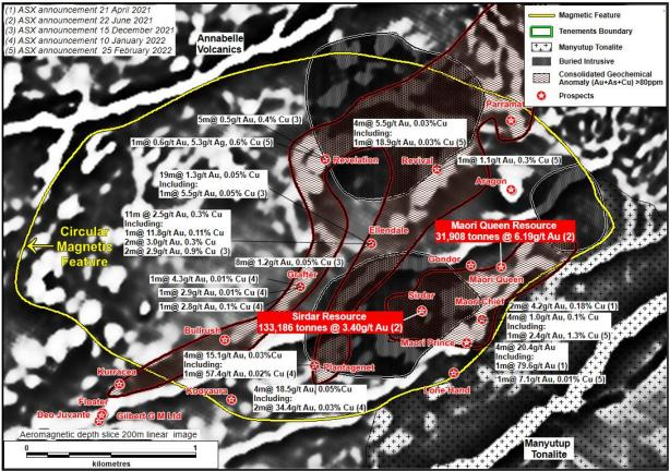
Figure 8. A grey scale aeromagnetic image showing the position of the buried intrusives within the intrusive complex (defined by yellow line), prospect and mineral resource positions, surface soil geochemical anomalism (Au, Cu and As) plus select peak drillhole intersection results.
