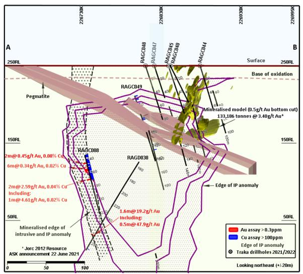
Figure 6. Cross-Section of the Sirdar Prospect showing the position of the IP anomaly associated with the Sirdar resource, the hanging wall mineralised structure and the intersections on it at the margin of IP anomaly.
