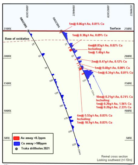
Figure 3. A cross-section of the mineralisation intersected at the Revival Prospect.
