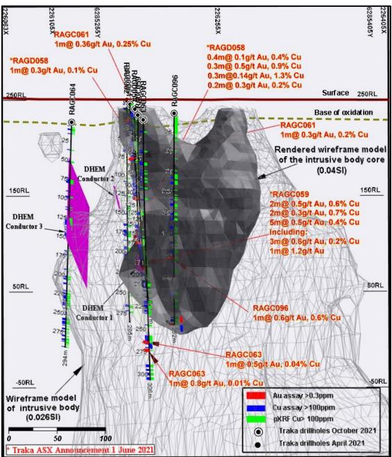
Figure 5. A long section view of Revelation showing the wireframe of the intrusive body, the DHEM conductors and drillholes with selective drillhole intersections.
