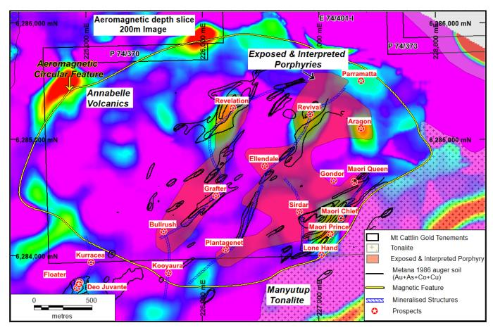
Figure 1. Aeromagnetic image of the Mt Cattlin Gold-Copper Project showing key prospects. The image shows the northeast trending gold soil geochemical anomaly extending over 1km between Plantagenet-Ellendale-Revival.
