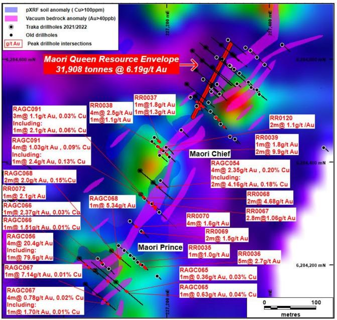
Figure 4. A resistivity image showing drillhole locations, anomalous gold soil geochemistry and peak drillhole intersections.
