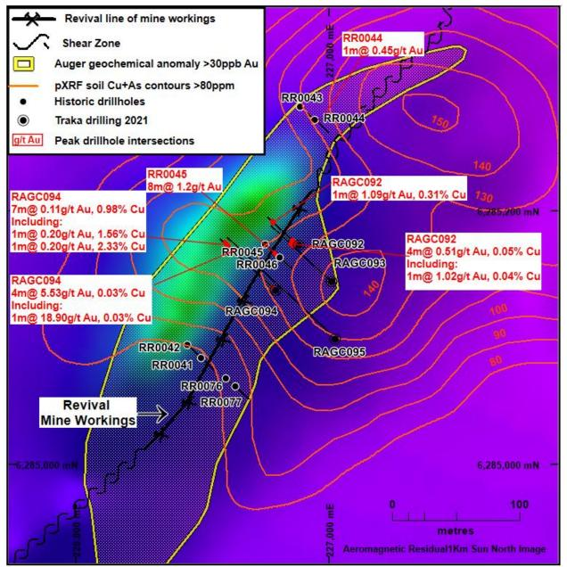
Figure 2. A plan view of the Revival Prospect showing historical and new drill hole locations on aeromagnetic image with geochemistry information draped over.
