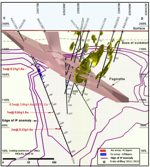
Figure 7. A cross-section of the Sirdar Prospect showing the position of the IP anomaly associated with the Sirdar resource and intersections down-plunge and within the IP anomaly.
